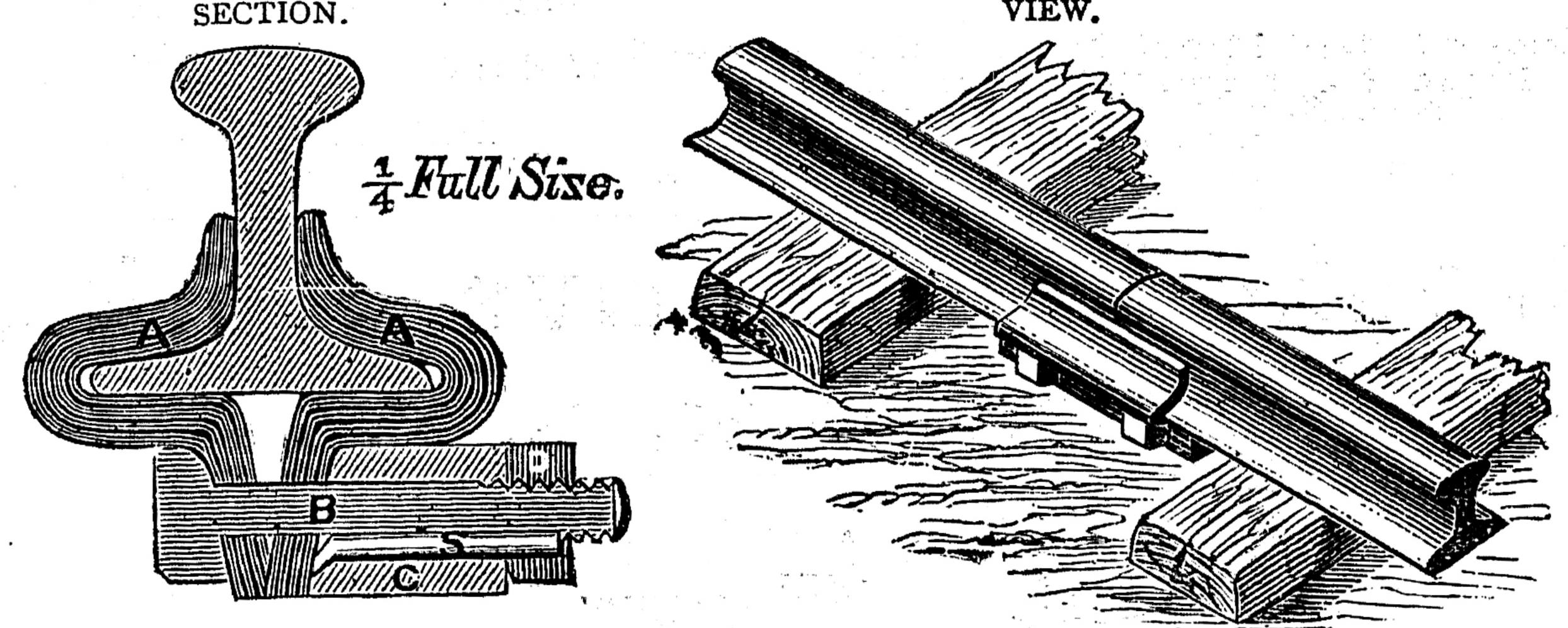
VIEW AND SECTION show position in place. A.—Is CLAMP-TRUSS. B.—Are two ¾ inch Bolts. C.—An Iron Collar, (a prepared wood block can be used in its place if parties prefer it.) D.—Is the Nut. S.—T'e LOCK of the NUT, which prevents its jarring loose.
